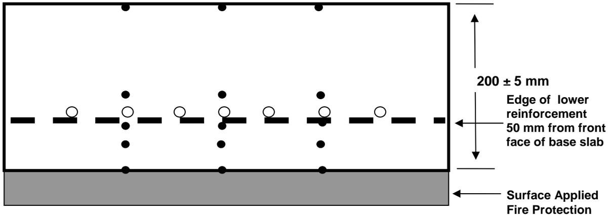
4 thermocouples located at: the protection interface (2, 4, 6, 8),
