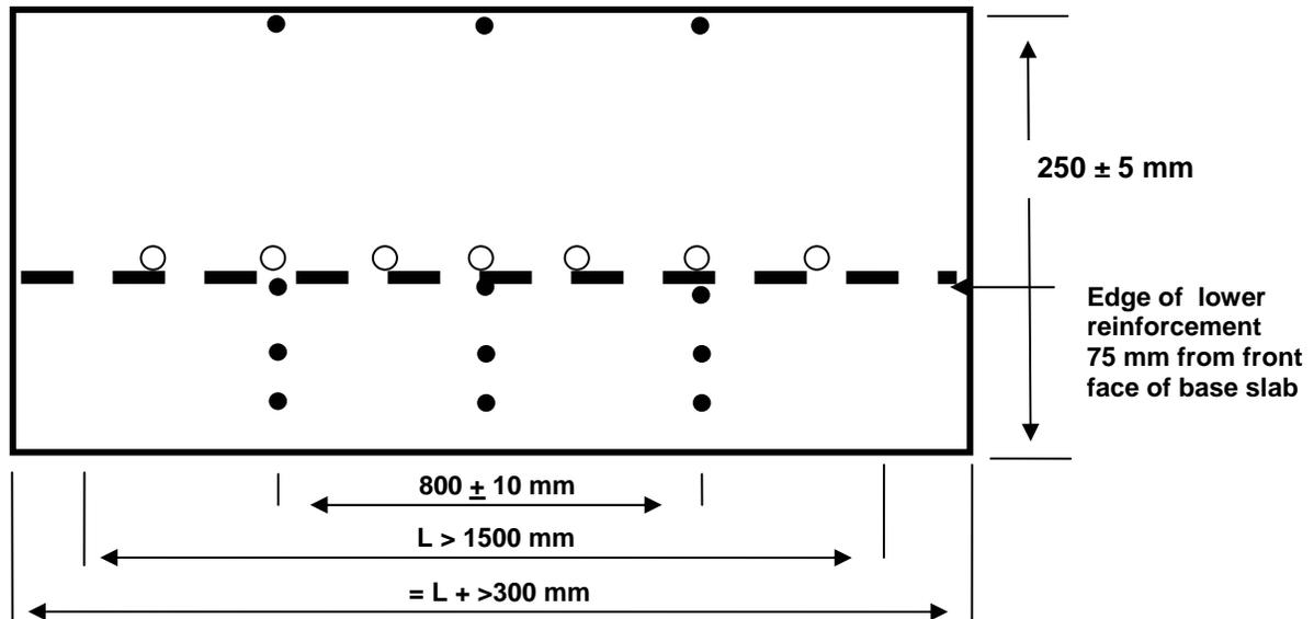
4 thermocouples 25 ± 2 mm the from the front surface of the concrete (2, 4, 6, 8),
