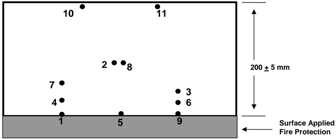
3 thermocouples located at: the protection interface (1, 5, 9), 2 at 25 ± 2 mm (4, 6), 2 at 40 ± 2 mm (3, 7), 2 at 75 ± 2 mm (2, 8), from the front surface of the concrete, plus 2 on the back face (10, 11).
