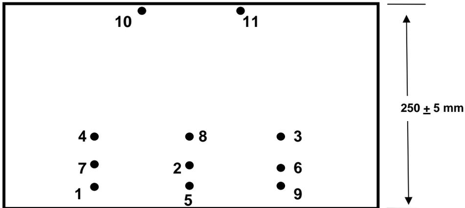
3 thermocouples located at: at 25 ± 2 mm (1, 5 & 9), 3 at 40 ± 2 mm (2, 6, 7), 3 at 75 ± 2 mm (3, 4, 8), from the front surface of the concrete, plus 2 on the back face (10,11).
