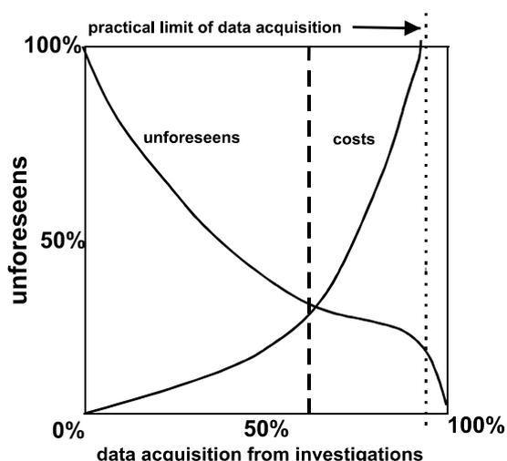
The amount of detail required during the site investigation will depend on the dimension and purpose of the tunnel, on its location, on the ground conditions and existing knowledge. The greater the volume of data acquisition, the lower will be the risk of uncertainties.
