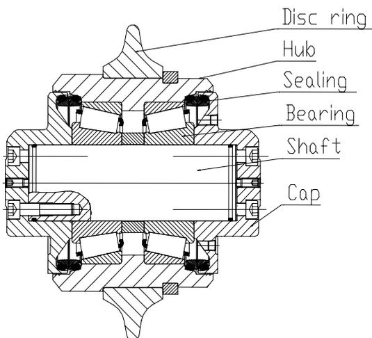
**Figure 15.3: Typical disc cutter design**
