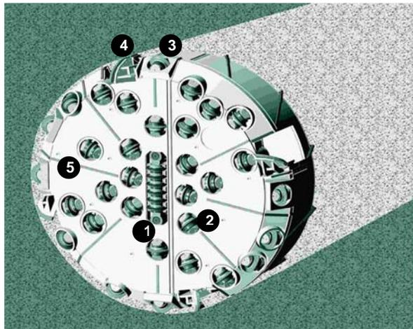
Figure 14.3: Cutter Head front view
