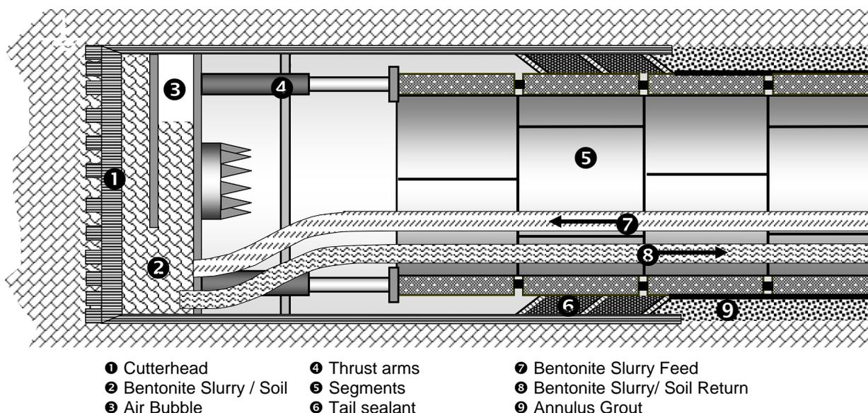
**Figure 9.1: Schematic Representation of Slurry Shield Machine**
