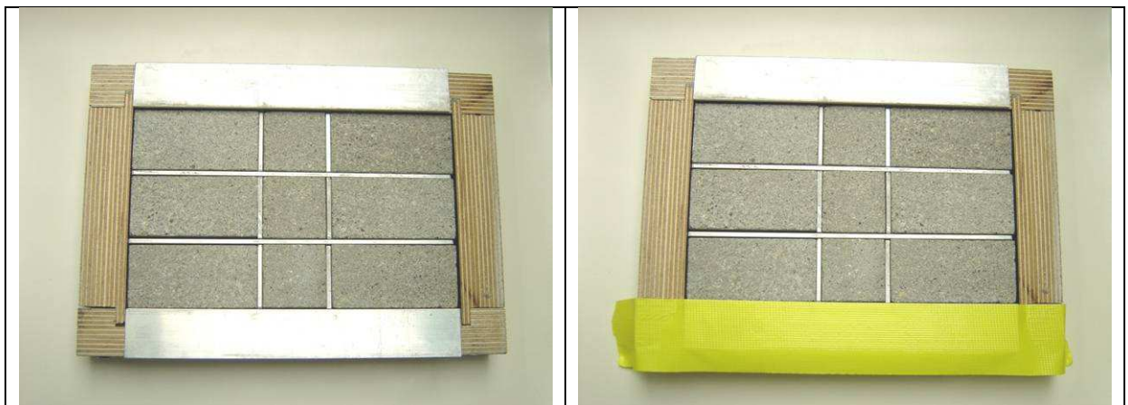
Fig. 4: Spacer Placing and Fixing
